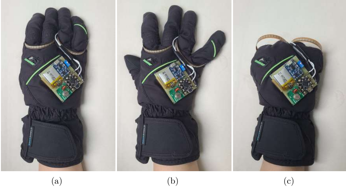
Figure 15.: The glove is shown in different positions. In the rest position (a), the flex sensors are bent more than in the spread position (b). In the fist position (c), the sensors have almost the same bend radius as in the rest position, but they are angled away from the glove.
