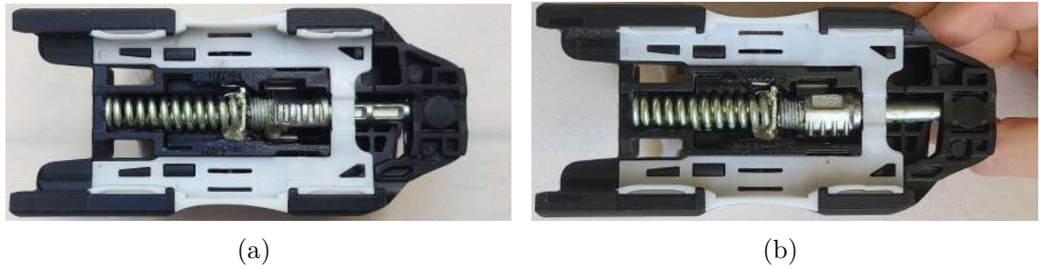
Figure 18.: Underside of the heel piece of the binding when detached from the track. The left image (a) shows the locked state. In (b) the lever is turned to open the interlocking teeth, so the heel piece can move back and forth along the rail.
