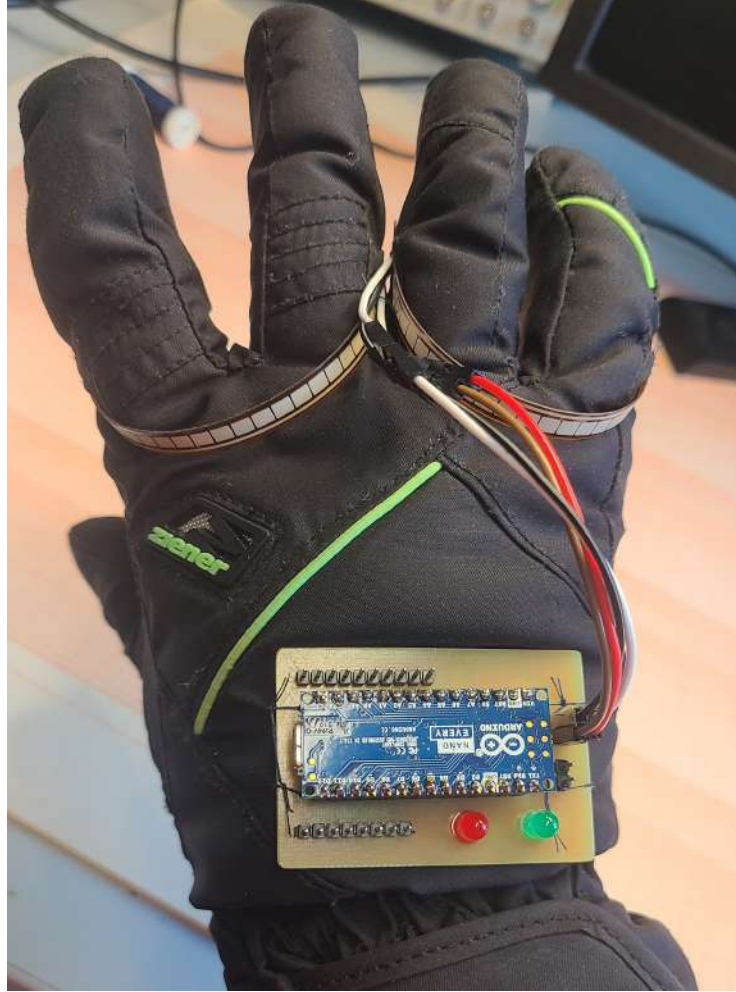
Figure 9.: First test setup of the flex sensor glove. Sewed onto the glove are two flex sensors and a circuit board housing an Arduino, two LEDs and voltage divider circuits for the flex sensors.
