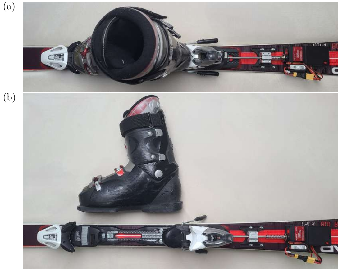
Figure 19.: The automatic binding release system together with the ski boot. In (a) the system is closed and the ski boot is attached. The system after release is shown in (b). The toe and heel piece are now too far apart to hold the boot in place.
