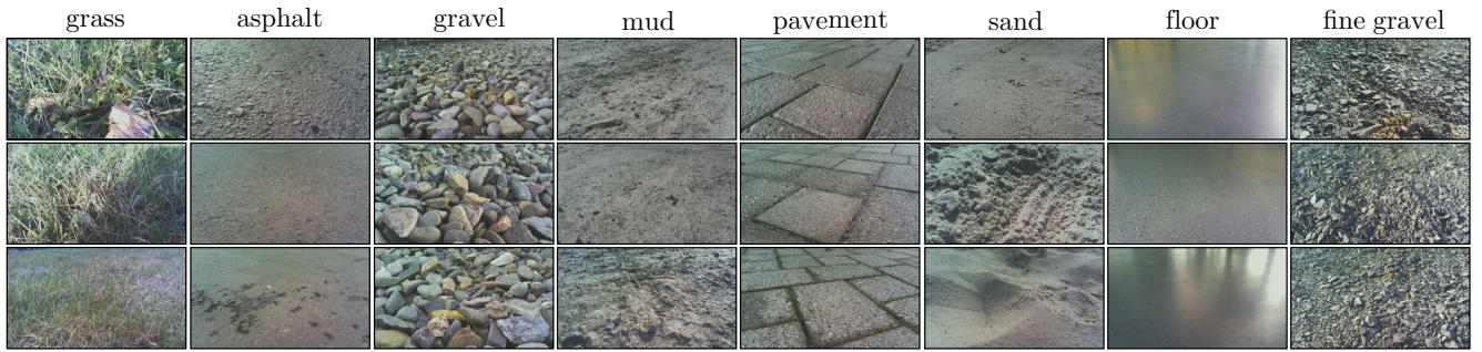
Fig. 5: Sample images from the terrain image set with eight different classes: grass, asphalt, gravel, mud, pavement, sand, floor, and fine gravel. Each terrain class has at least 80 samples taken under different lighting and weather conditions.
