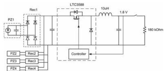
Figure 4: PZT Energy harvesting circuit diagram
