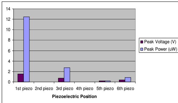
Figure 11: Peak voltage and peak power at 6 MFC locations
