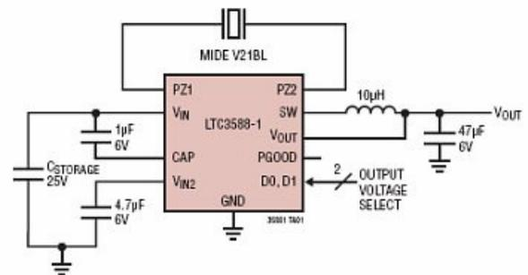
Figure 5: MFC Energy harvesting circuit diagram
