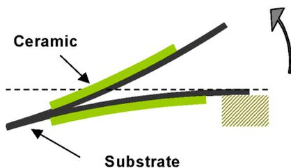
Figure 2: Diagram of the PZT piezoelectric
