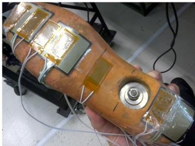
Figure 8: MFC installing in the prosthesis foot
