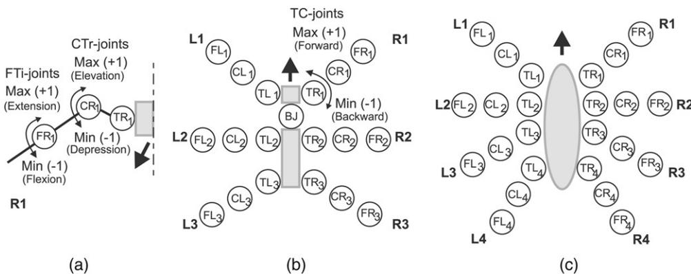
Fig. 5. (a) The movements of the CTR- and FTI-joints of the right front leg ( $R_1$ ) with the remaining legs of both machines performing the same (front view). (b) The location of the motor neurons on the AMOS-WD06 and the movements of the TC-joints. (c) The location of the motor neurons on the AMOS-WD08 where the movements of the TC-joints are similar to those of the AMOS-WD06.
