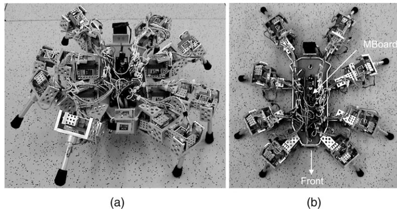
Fig. 2. The physical eight-legged walking machine AMOS-WD08. (a) Front view. (b) Top view.
