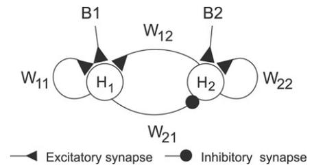
Fig. 6. The 2-neuron oscillator network.
