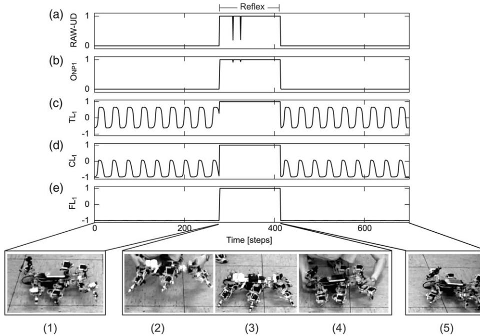
Fig. 21. (a) Raw-UD signal. (b) Preprocessed UD signal. (c)–(e) Motor neuron signals of the TC-joint ( $TL_1$ ), CTr-joint ( $CL_1$ ), and FTi-joint ( $FL_1$ ) of the left front leg, respectively. Signals of other joints having similar patterns to those of the left front leg are not shown. A series of photos of the reflex behavior is shown below. The video clip of this experiment can be seen at <http://www.nld.ds.mpg.de/~poramate/RAS/Reflex.mpg>.
