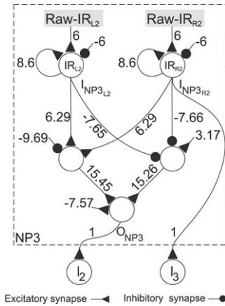
Fig. 19. Neural preprocessing unit  $NP3$  of the IR signals  $IR_{R2,L2}$  (dashed frame). It is created as an XNOR network with a self-connection at its input neurons. As a result, the input neurons function as hysteresis elements, the effect of which is similar to that shown in Figs. 18(d) and 18(f). The output of the network  $o_{NP3}$  is fed to  $I_2$  and the output of one hysteresis element  $I_{NP3,R2}$  is connected to  $I_3$  (see text for details).
