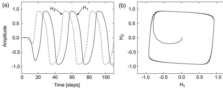
Fig. 8. (a) The sinusoidal output signals from the neural oscillator network where the parameter set is:  $B_1 = B_2 = 0.01$ ,  $W_{21} = -0.4$ ,  $W_{12} = 0.4$  and  $W_{11} = W_{22} = 1.5$ . The update frequency of the network is approximately 25 Hz. (b) The phase space with the quasi-periodic attractor of the oscillator network.
