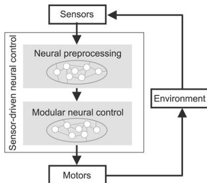
Fig. 17. Diagram of sensor-driven neural control. The controller acts as an artificial perception–action system, i.e., the sensor signals go through the neural preprocessing modules into the modular neural control module (compare Fig. 4) which commands the actuators. As a result, the robot's behavior is generated by interacting with its environment in a sensorimotor loop.
