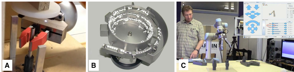
Fig. 2 a Specialized gripper for a specific assembly task with a specific object. b Typical feeding machine used in automated assembly. c Control panel based programming of the UR robot arm
