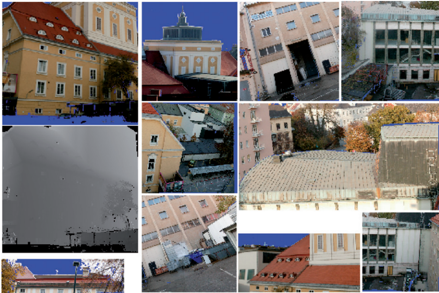
Figure 5. 10 of the 20 3D data sets used in the analysis. The points without range information are marked in blue. The gray image shows the range data of the top-left scene.
