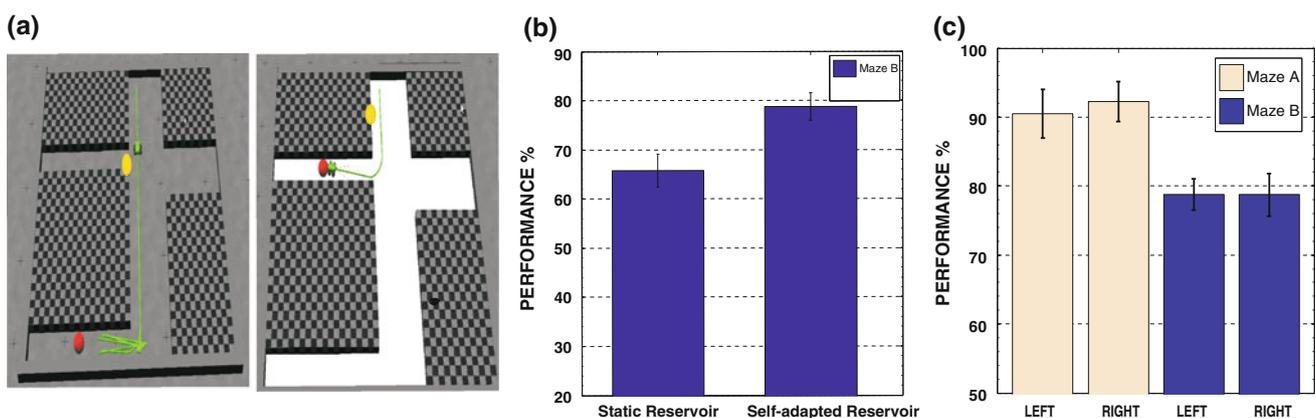
**Fig. 6** a Screenshots of the robot successfully navigating through the long maze B (left) and the short maze A (right). Yellow ball is cue to turn right at the T junction, red ball marks delay time between cue and the recall zone. b Performance on the large maze B simulation task after 80 trials for static reservoir versus our self-adapted
