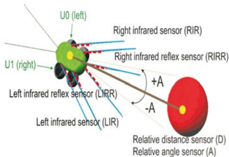
**Fig. 4** Model of the simulated wheeled robot NIMM4 showing the sensors (LIR, RIR, LIRR, RIRR) and actuators (U0,U1). The red ball in front of the robot represents its goal
