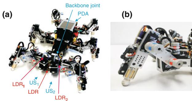
**Fig. 5** a Biologically inspired six-legged walking machine AMOS II. b Leg structure of AMOS II inspired from a cockroach leg (showing the three different leg joints) (color figure online)
