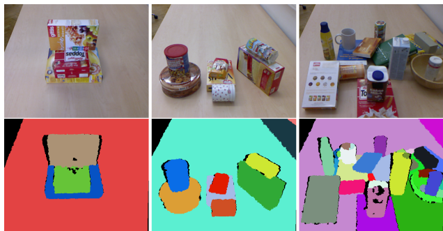
Figure 4. Example results for the OSD dataset. Points beyond a distance of 2m were cropped for visualization. Parameters: R_{\text{voxel}} = 0.005 , R_{\text{seed}} = 0.02 , \beta_{\text{Thresh}} = 10^\circ .
