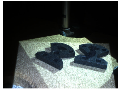
Fig. 2 A view of the real platform containing a subset of the Cranfield objects, with a texture projection for better stereo reconstructions
