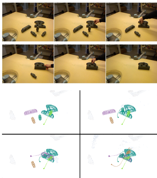
Figure 9: Tracker results for a complex assembly sequence. The bottom images show the tracked object models, represented by point clouds, at the key-frames which are also shown in the four intermediate top images.
