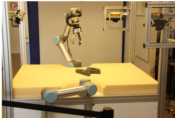
Figure 2: The robotic MARVIN platform with two manipulators and three camera pairs.
