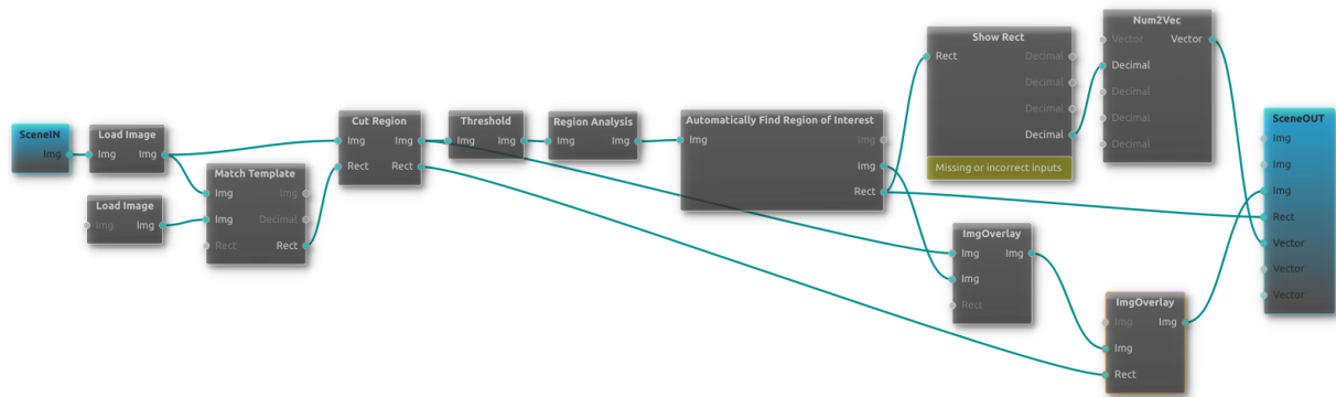
Figure 3: Graph view of the algorithm diagram editor. Each block contains a “configure” dialogue, which allows setting properties of the block.
