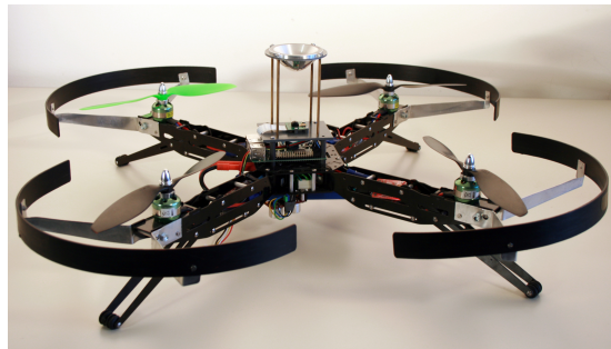
Figure 1: The quadrocopter utilized in this work. In the center, a camera captures omnidirectional images via the mounted mirror (Compare Fig. 3a).
