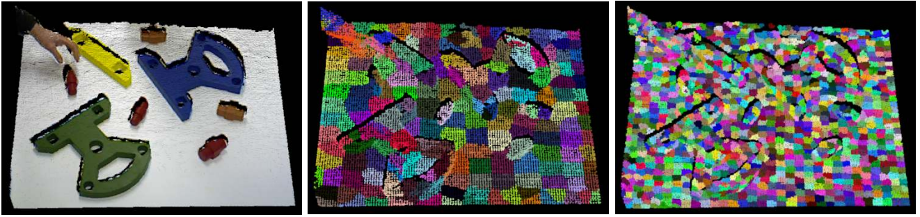
Fig. 1. Supervoxels found using VCCS. From left to right: original RGB image, supervoxels with R_{seed} = 0.08\text{m} , and supervoxels with R_{seed} = 0.03\text{m} .
