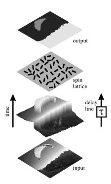
Figure 1: Schematic diagram of the system. The input image is piped into a luminance-dependent delay line. Bright objects are processed before dark objects. The temporal structure of this data stream determines the interaction between spins within the second part of the system, which consists of a spin lattice.
