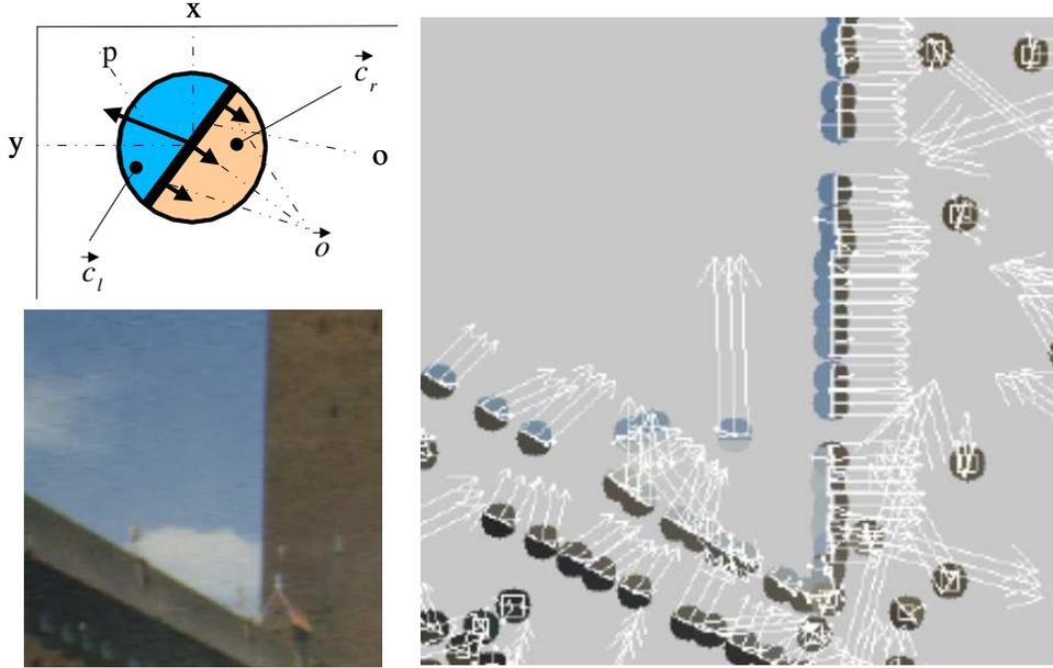
Figure 2: **Top left:** Schematic representation of a basic feature vector. **Bottom left:** Frame in an image (the frame is part of the image sequence shown in figure 3 left). **Right:** Extracted Feature vectors.
