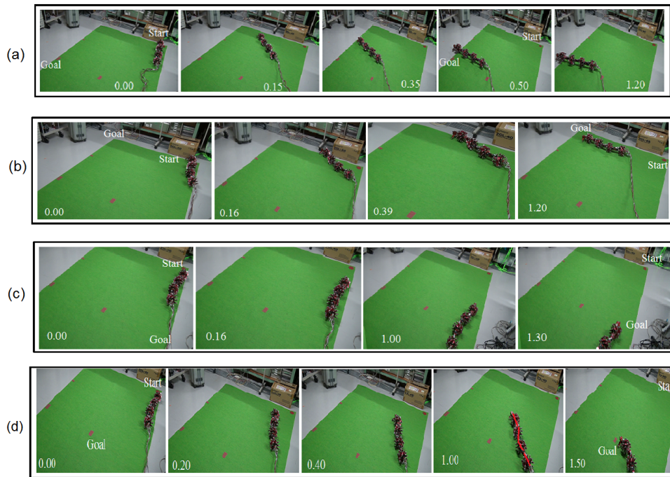
Figure 8. Experiment 5: Generating new behaviours with parameter interpolation. Start position is (0m, 0m). (a) Primitive P_{1_s} from the library. It is generated using the goal (2m, 2m) for a straight-line shape. (b) Primitive P_{12} from the library, which is generated using the goal (0m, 2m) for a semi-zigzag shape, having \phi_1 = 0.5\text{rad} , \phi_2 = -0.5\text{rad} , and \phi_3 = -0.1\text{rad} . (c) Primitive P_{13} from the library, which is generated using the goal (2m, 0m) for a semi-zigzag shape. (d) The robot reaches the goal (2m, 1m) using parameters obtained by interpolating the above primitives belonging to different robot shapes.
