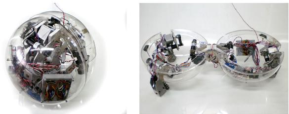
Fig. 1. A Reconfigurable Spherical Robot
