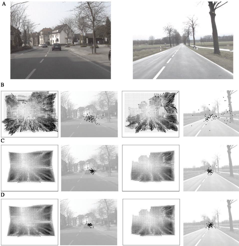
Figure 2. A: First frames of the camera sequences for different driving scenarios, left: town sequence, right: road sequence. B: Raw optic flow estimated from the first three frames by the Lucas – Kanade algorithm and heading estimates computed from 100 random sub-samples of the flow field. The black cross marks the principal point. The small boxes marks the singular heading estimates. The large boxes marks the mean heading estimate of the 100 runs. C: Flow fields and heading estimates after constant filtering. D: Flow fields and heading estimates after space-variant filtering.
