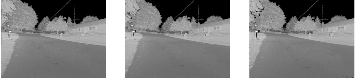
Figure 5: Three image frames selected from a sequence generated from the brid-data. The first image is the first of the sequence, the following images have a distance of 15 and 30 frames respectively from the first. The simulated self movement results in a translational shift of 0.01m and a rotation of 0.01 degree per frame. The ratios between width and height and the focal length are chosen as 1 and 0.7 respectively.
