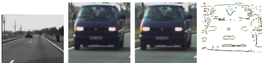
Figure 11: IMO processing. (a) IMO list and BBs (b) left image segment, (c) right image segment, (d) extracted primitives and stereo correspondences.
