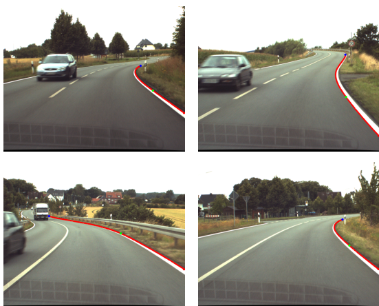
Figure 9: Extracted right lanes (shown in red) for some images in the reference sequence.
